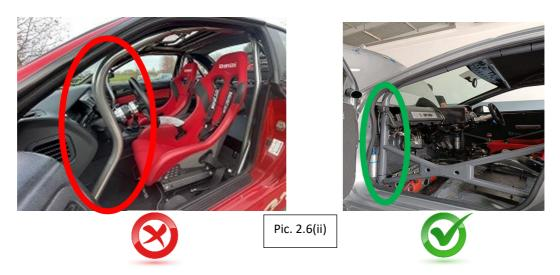
Should removable members be used in the construction of a safety cage, the dismountablejoints used must comply with a type under FIA Article 253.
